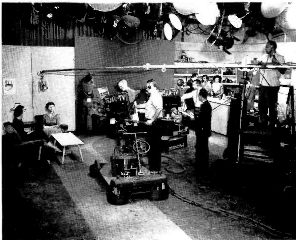
Studio A — The "Big Studio" shown on the air, with next program in sight being set up. Studio A has 3 RCA RK10A studio cameras. Complete lighting equipment includes Kliegl dimming control panel to light nearly 100 linear feet of sets. Contains modern electric kitchen and many other basic sets. Production staff available for consultation with clients. Studio B has its own camera and set facilities.
