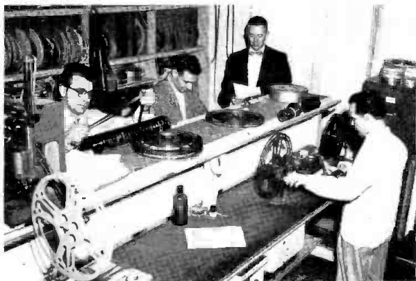
Channel 10 Film Room — Film Director Bill Cooper receives and logs in all films — inspects, screens, times, edits for use on the air. He presides over two RCA 16 mm projectors, two automatic selectro-slide projectors, an SVE strip film projector, a Gray Telop opaque projector, rear screen projector and a TDC slide projector — all used in conjunction with two RCA TK20A film cameras with latest improvements. 16 mm cameras, Speed-graphic and instantaneous Polaroid cameras, plus completely equipped laboratory for rapid processing stills and motion pictures are in constant use.
